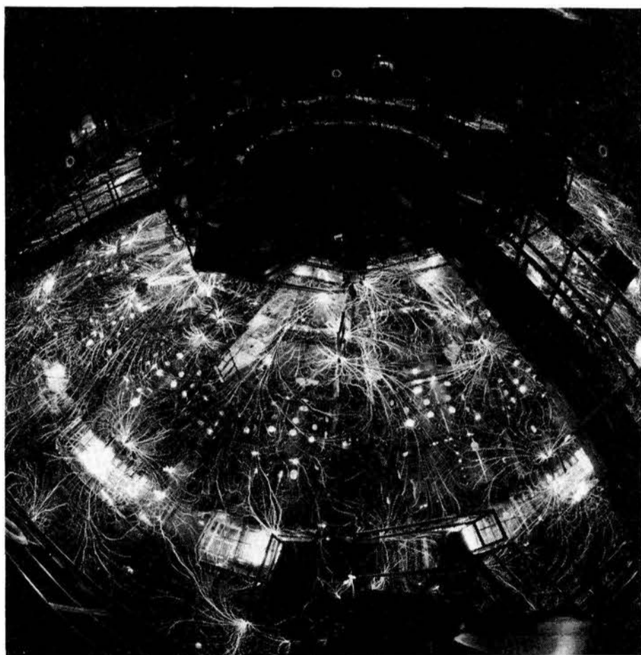
JUST SHOCKING — Surface electrical flashovers put on spectacular display during test firing of the Particle Beam Fusion Accelerator (PBFA II).
